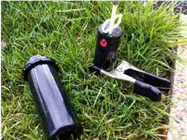
Clamp used to hold sprinkler in UP position for adjustment.
